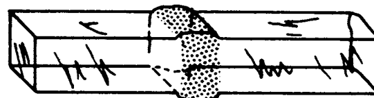
Joint "drying." Cushions harden.
